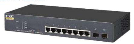
NS2010VPEL is the web-based Smart PoE Switch which has PoE 8 ports of 10/100/1000BASE-T and 2 slots of 100/1000BASE-X. This PoE switch supports IEEE802.3af/at and can supply 30w per port and is provided with the max 75w budget in entire PoE system.
