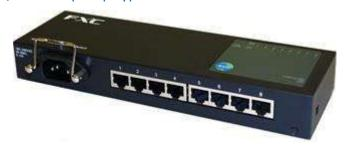
Each port supports auto-negotiation, enabling automatic setting of the transfer speed, transfer method, and polarity of each port.
